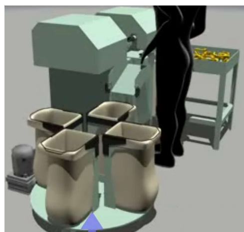
Automatic Rotary Packer Rotating at Pre-set processed amount
