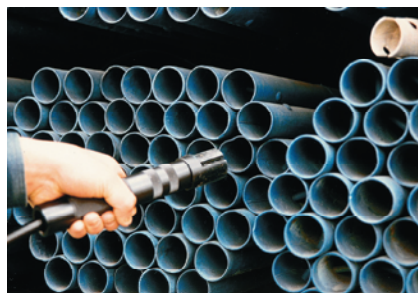
φ48.6 mm straightening jig
