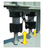
■Dual-jack design laminates need to turn over steel planks.
