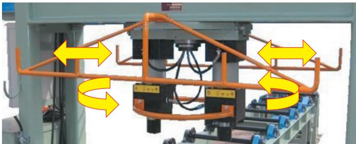
■ The jack swings and shifts, enabling it to quickly and reliably secure the target plank (manual operation).
