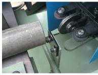
Cutting blades are made of commercially available super-hard metal to facilitate long-term usage and easy replacement.
