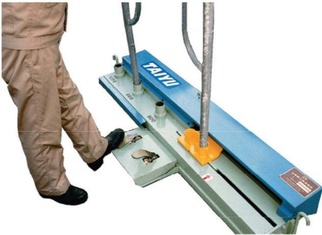
Frame width is easy to adjust (foot-operated).
