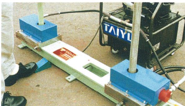
Punching is made at the touch of a button correctly. Frame width checks (width·inner diameter of pipe) are made simultaneously with punching at the touch of a button.
